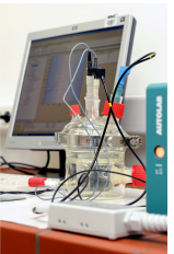
Example of corrosion potential measurements of different coatings on patinated bronze in artificial acid rain
